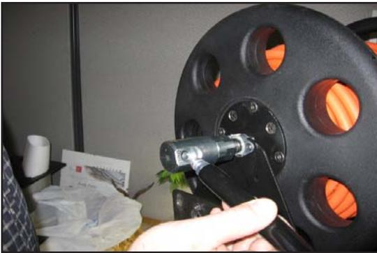
**Figure 2-24. Install Hose End into Swivel**
