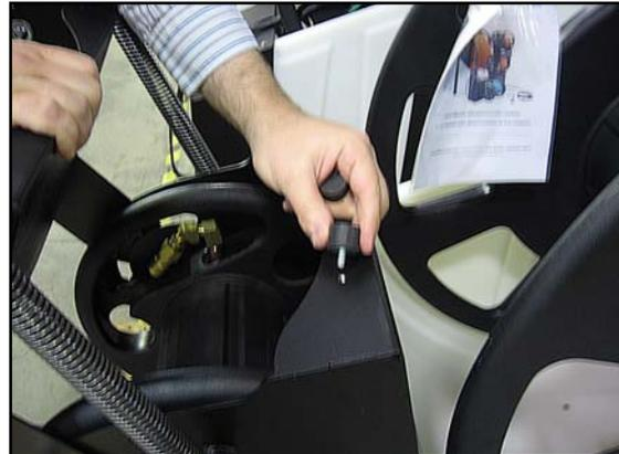
**Figure 2-36. Install 2 Rubber Mounts**
