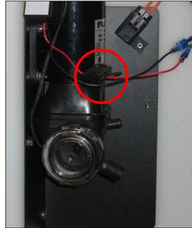
**Figure 7-1. Remove 15 Amp Fuse from Fuse Holder**
