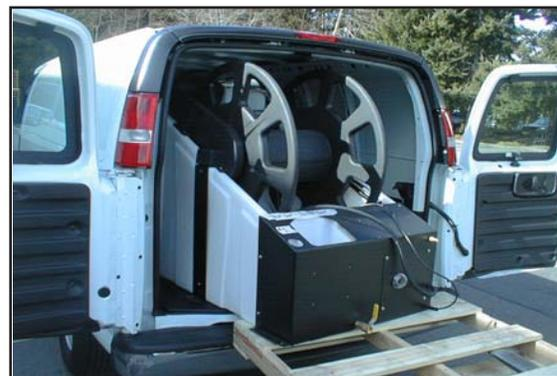
**Figure 2-2. Load Tank into the Van**
