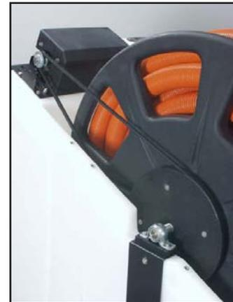
Figure 7-3. Belt Cover Removed
