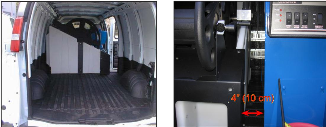
**Figure 2-4. Position Tank Parallel to Cleaning Unit; Space between HydraCradle Tank and Cleaning Unit Should Be 4" (10 cm)**
