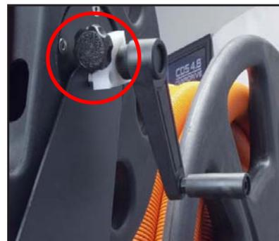
**Figure 2-21. Turn Tension Knob to the Right to Set Brake**
