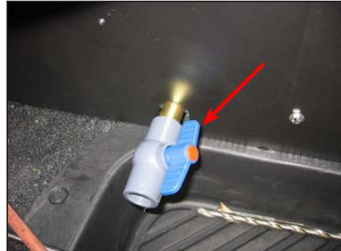
**Figure 3-1. Turn Drain Valve**
