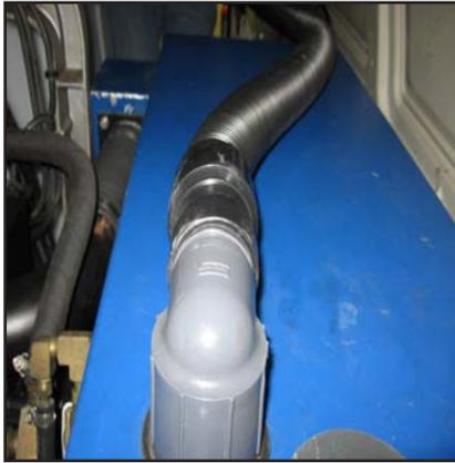
**Figure 2-17. Connect Recovery Tank Hose into Cleaning Unit's Tank Cuff**
