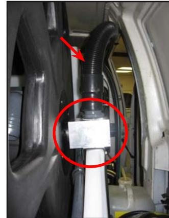
**Figure 7-7. Remove Recovery Hose from Live-Center Mount**
