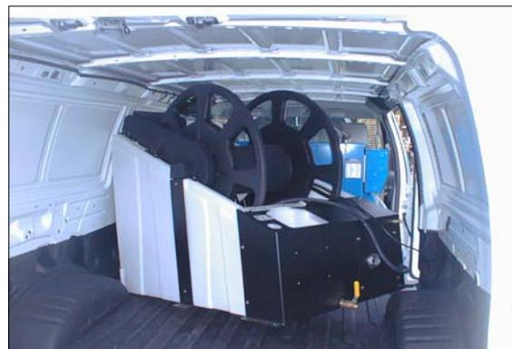
**Figure 2-3. Pivot Tank over the Wheel Well**
