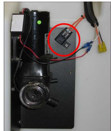
**Figure 7-2. Remove 30 Amp Fuse from Fuse Holder**
