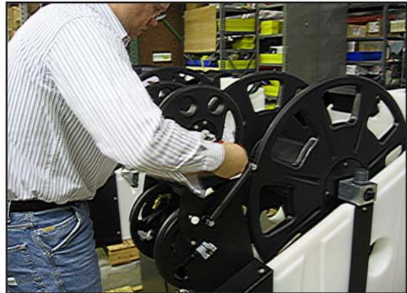
**Figure 2-37. Secure 1st Hose Reel to Bracket**
