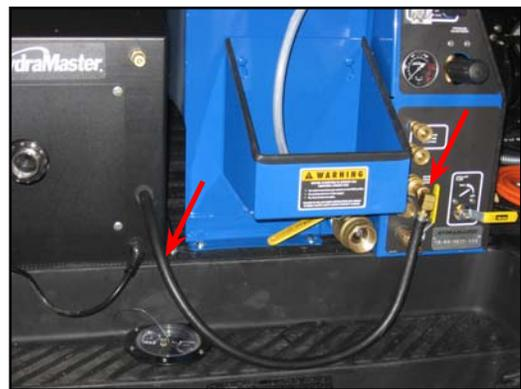
**Figure 2-15. Connect Pump-in Pump Hose**
