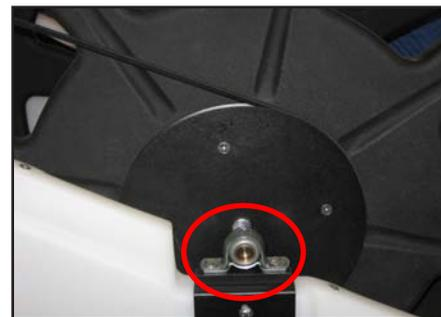
Figure 7-5. Remove Pillow Block Bearing
