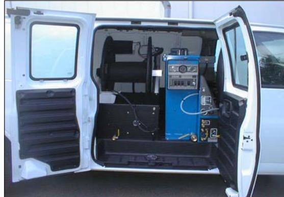
**Figure 2-1. Sample Configuration of HydraCradle Tank Installation with CDS Unit in GM Van**
